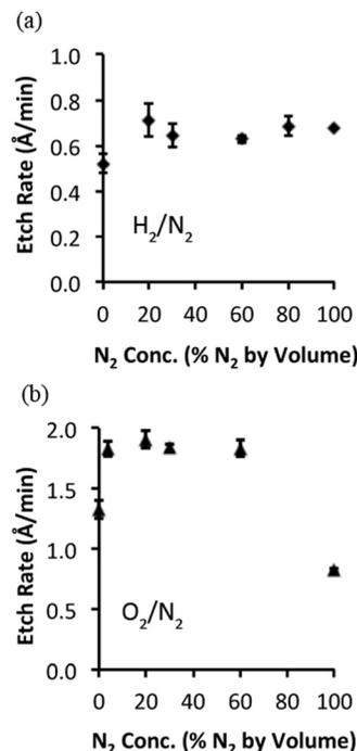
FIG. 3. Si<sub>3</sub>N<sub>4</sub> etch in remote (a) H<sub>2</sub>- and (b) O<sub>2</sub>-based plasmas. Etch rate was measured as a function of varying N<sub>2</sub> concentration while fixing the temperature at  $T = 300$  °C and keeping the total flow rate constant. The error bar represents the standard deviation of the etch-rate measurements.
